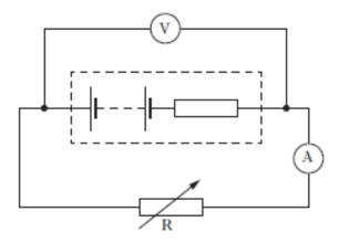
The variable resistor R is adjusted and a series of readings taken from the voltmeter and ammeter.
