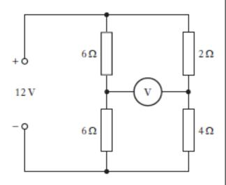
The reading on the voltmeter is
